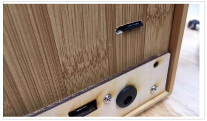
HINT: If you have loaded the disk images on the card and see nothing but a non-stop sequence of "c" when you access the card, you need to completely reformat the card (FAT or FAT32, be sure to select FULL format, not a quick format.)
