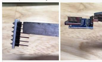
Install the module with the SD card holder facing toward the outside of the PC board, or toward the hole cut for the port as shown. Make sure it is perpendicular and square with the PC board. I find it best to place the module in the hole in the case, then place the PC board over it before soldering. This makes sure the distance between the module and the PC board is correct.
