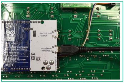
It's time to put the completed circuit board into the case. You will have to gently push down the connector for the serial module to slightly bend down the pins. Also note the orientation of the USB extension cable, this will keep it out of the way of the PC board.
