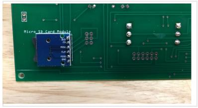
If you would like the micro SD card accessible from outside the case, take a needle-nose pliers and carefully bend the pins to a 90 degree orientation.
