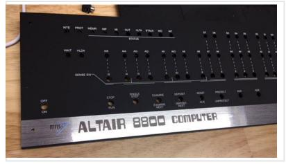
Put the front panel in place, push down around the LEDs and switches to set it properly, and add the 10mm nylon bolts.
