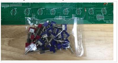
Put all the switches in place without soldering them. 17 two position toggles on the top row and the power switch location, 8 three position momentary toggles on the bottom row.
