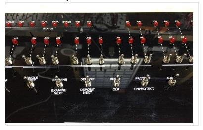
While you are soldering the LEDs, you can verify that the long lead is toward the bottom of the board.
