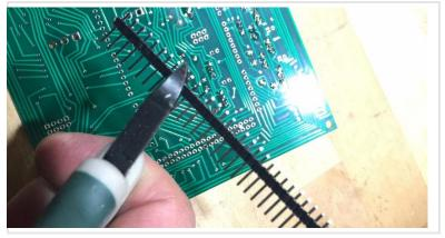
Add the male headers to the <u>underside</u> of the PC board. You can also add the six-pin female header for the SPI connector on the Arduino. Make sure you add these to the correct side of the board because desoldering 92 connections would not be fun!
