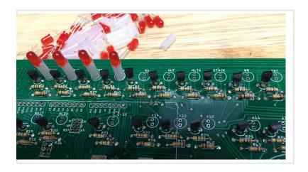
Again, like the switches, put the front panel in place to hold the LEDs while you solder them.
