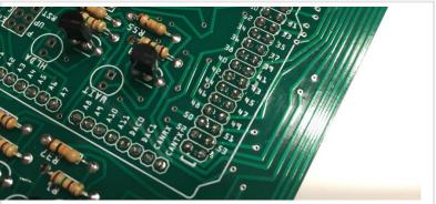
After you're done soldering the headers, try putting the Arduino in place and check for a secure fit. Remove it when you're done.
