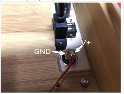
Solder the other ends to the power input on the opposite side of the PC board. Make sure there are no shorts, and that you don't reverse the polarity.
