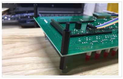
On the other side add the 14mm male/female standoffs on the top, and two 20mm female/female standoffs on the bottom.
