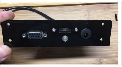
Attach it in place to the bamboo case with the bottom two screws only (with washers and nuts).
