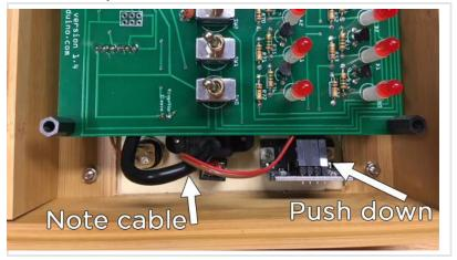
If you put the SD card in before you do the final assembly, it will help you guide the SD module into place in the slot you cut in the case.
