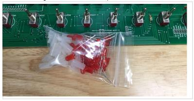
Just like the switches, put the LEDs and spacers in place and do not solder them. You do not have to do them all at once, it may be easier to do them in two or three groups. The orientation if the LEDs is crucial. Make sure the long lead of the LED is toward the bottom of the PC board and the flat side of the LED is toward the top.
