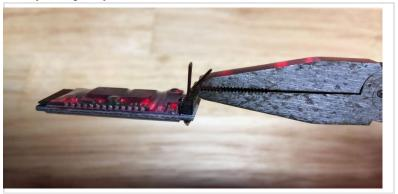
You can now solder the Bluetooth module to the *underside* of the PC board.
