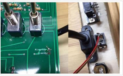
Next, we connect the serial port module to the PC board. You should have part of the Arduino header left over, so solder a four pin segment to the underside of the PC board – this is where the cable will plug in. The pins are labeled on the top of the PC board and on the serial module.
