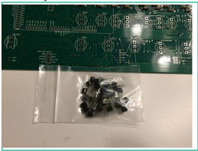
The orientation of the transistor is crucial, but relatively simple. Just make sure the flat end of the transistor is facing up, just like the image printed on the circuit board.
