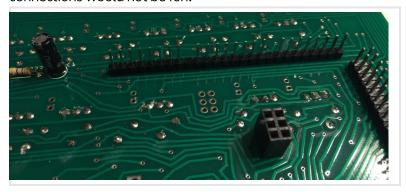
Solder the headers carefully. Make sure they are as close to vertical as possible, and make sure the solder flows completely over the connection. **Most problems happen** here with cold solder joints, or solder bridges.
