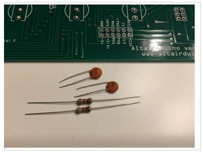
Those can be mounted on the front of the PC board in R74, R75, C2, and C3 on the lower right side of the board. The orientation of the components does not matter.
