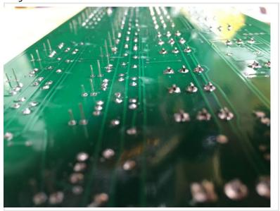
Make sure you trim the leads after you solder the components. Next, we are installing a ribbon cable that could get punctured if you leave the LED or transistor leads untrimmed.
