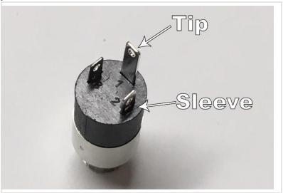
Wire the sleeve connection through both pins 2 and 3 on the round connector.
