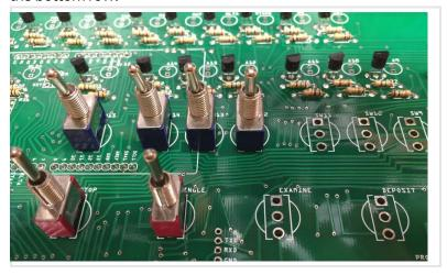
Put the front panel in place to hold the switches in the correct position (having all two-way switches in the down position makes this easier.)
