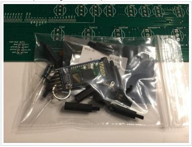
In that bag you will find one electrolytic capacitor and one  $470\Omega$  resistor (Yellow, Violet, Brown, Gold color code). If you don't want to decipher the color code, just know you will find three resistors in the bag, two that match, and one that does not. This is the one that does not match another.
