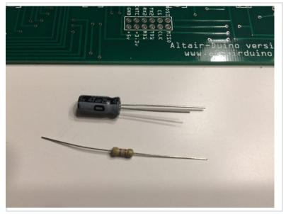
These two components mount in the back (underside) of the PC board in R73 and C1. The orientation of the resistor does not matter, but make sure the short lead of the capacitor (marked with a "-" on the side) goes in the hole also marked with a "-".
