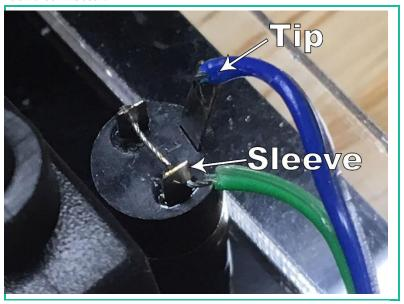
Audio jack connects to the opposite side of the PC board as the power connections.
