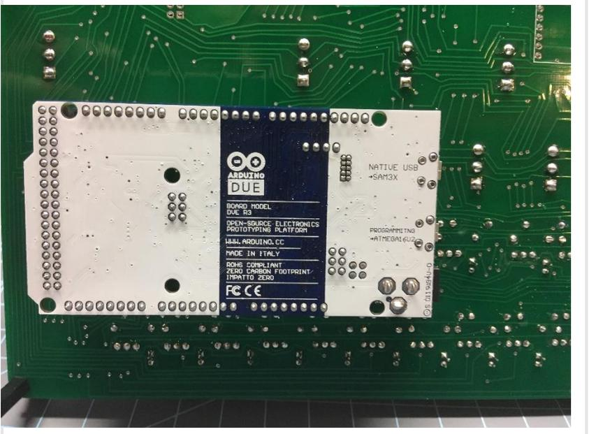
Get the main circuit board and solder a fourteen pin dual header on the lower right.
