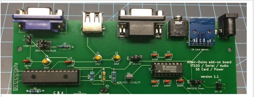
Add the required jumpers to the I/O expansion. The following are the "default" jumpers. Later you can read more about the jumper options on the website.
