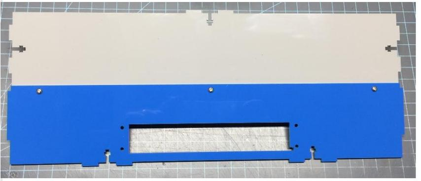
Attach the I/O circuit board to the blue bottom piece with four 8mm standoffs, nylon nuts and nylon bolts.
